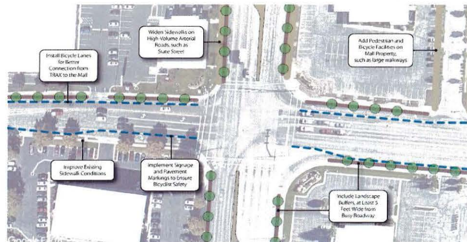
Figure 4.7 The intersection of State Street and Winchester Street currently lacks a safe bicycle experience. Future improvement recommendations include better bicycle lane signage as well as sidewalk improvements.
