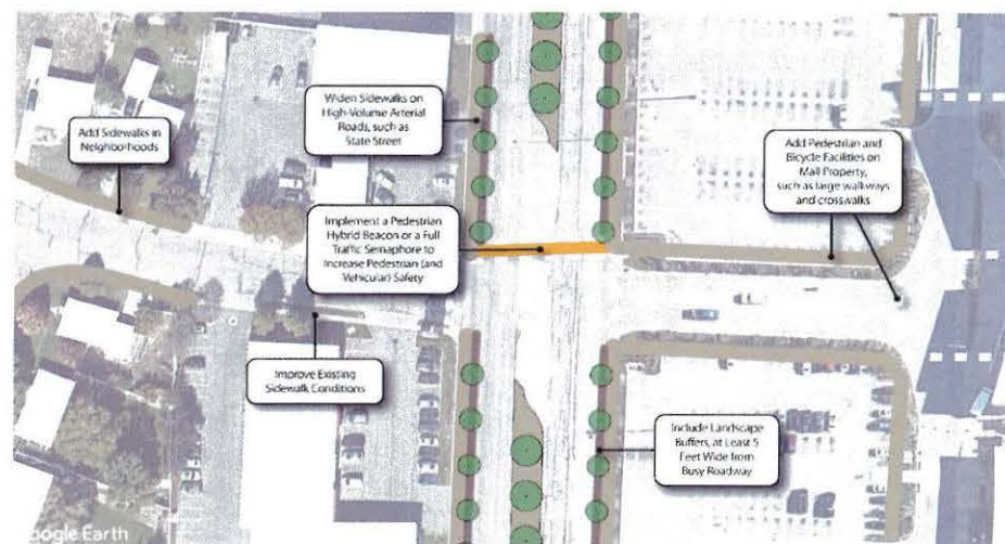
Figure 4.8 The existing intersection at Creek Road and State Street is lacking pedestrian amenities. Improving this intersection will increase connectivity from the neighborhood to Fashion Place Mall.
