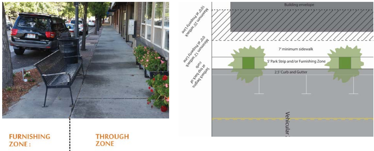
Figure 3 – MCCD required improvements include: 7' pedestrian zone, 5' furnishings zone
