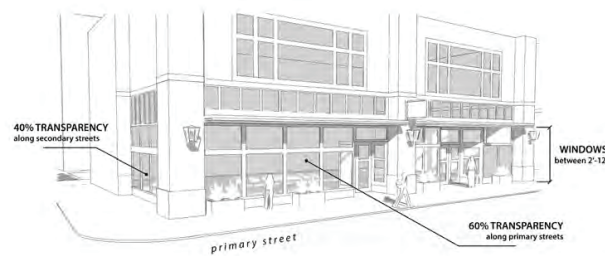
Figure 5.20 The diagram above visually illustrates transparency requirements. Height, width, and location of windows largely contributes to appropriate percentages of transparency.
