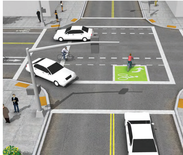
Figure 4.10 The FHWA outlines a two-stage bicycle turn box design similar to the ones implemented along 200 West in Salt Lake City which could be implemented at the Winchester and State intersection (image source: NACTO).
