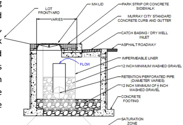
Figure 1. This diagram shows the major design components of this BMP. The Dry Well box captures the runoff, and the connected perforated pipes distributes it below park strips or sidewalks to be infiltrated into the underlying soils. The roadway and dry well box are maintained by the City and the property owner maintains the park strip as typical.
